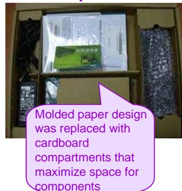
The taskforce also assessed packaging of peripheral products and standardized the packaging to four different sizes. The space for largest components was greatly reduced, for example the packaging depth for optical hard discs was cut from 110mm to 55mm.
